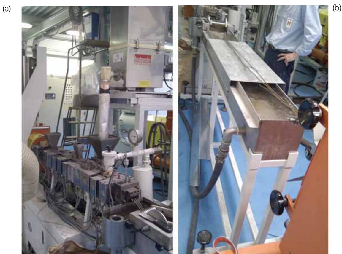
Figure 4.7: A typical compounding line: (a) overview and (b) strand granulation detail
