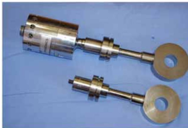
Figure 2.2: Complete 3 kW transducer stack
