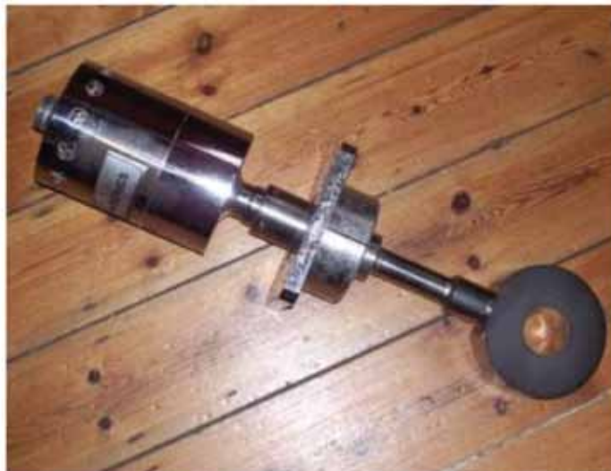
Figure 2.18: A single 6 kW fan cooled ultrasonic head comprising transducer, booster, extension and radial cell horn
