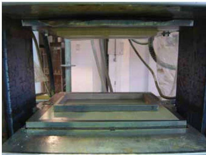
Figure 3.24: Specially designed mould for making SMC test specimens, fixed in hot press
