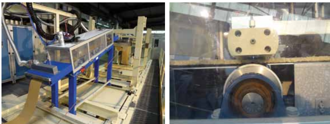
Figure 3.29: Pilot scale plasma unit of 25 cm wide (left), treatment of natural fibre non-woven (right)
