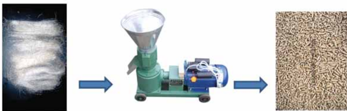
Figure 4.3: Turning loose fibres to fibre pellets by using a pellet mill
