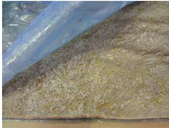
Figure 3.30: Protecting film released from SMC sheet, showing distribution of resin paste on hemp mat
