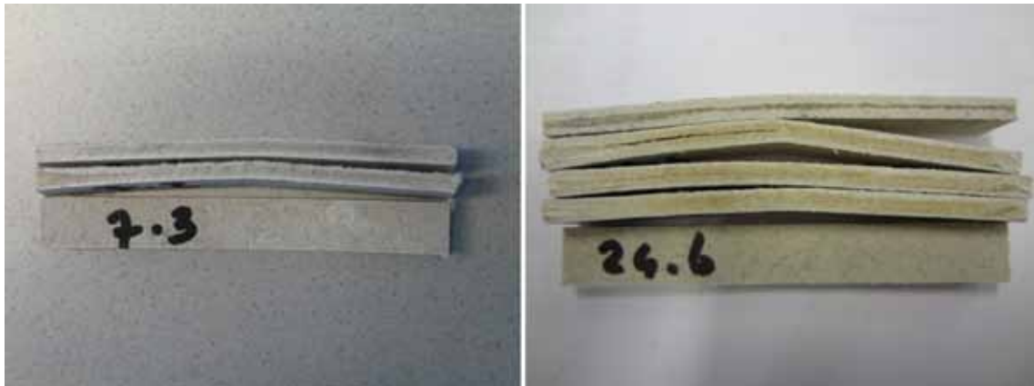
Figure 3.27: SMC specimens based on steam exploded flax fibre, the central section of the composite showing incomplete fibre impregnation. SMC-7 (left), SMC-24 (right)
