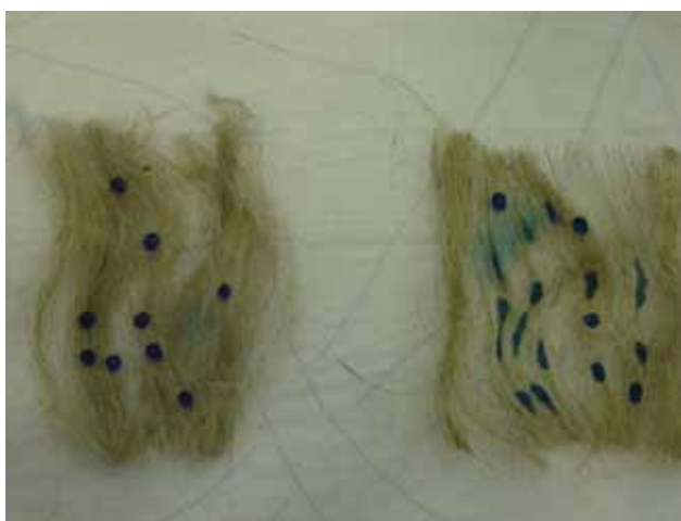
Figure 3.12: Water absorption increases after plasma treatment (right) compared to untreated reference (left)
