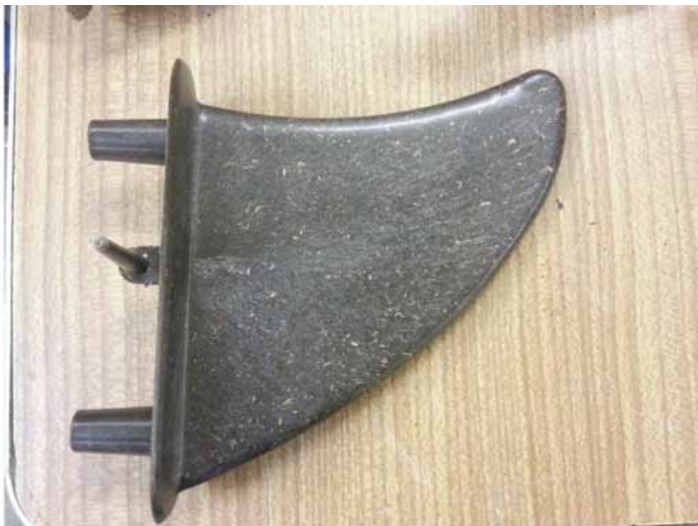
Figure 4.13: Typical injection moulding surfboard fin made from the best performing ultrasound treated hemp/PP compound
