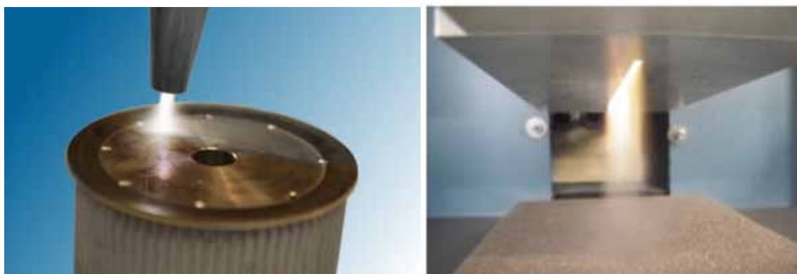
Figure 3.3: APP systems: nozzle type plasma source, also called ULS (left), slit type plasma source, also called ULD (right)
