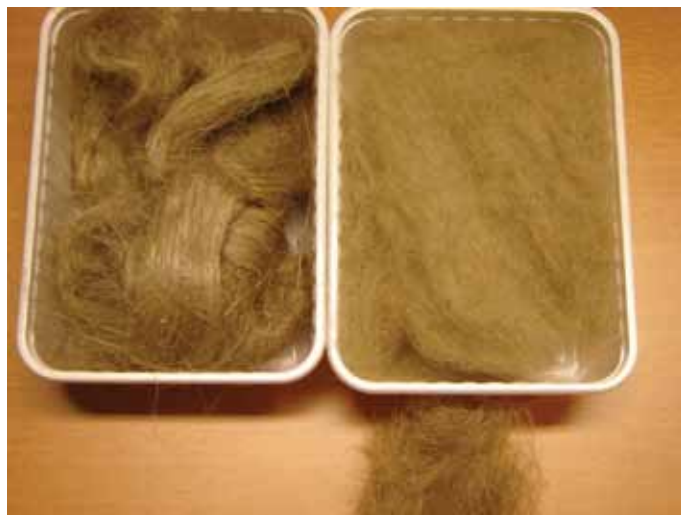
Figure 3.14: Shirley refined flax sliver: unrefined fibre (left), fine fibre (top right) and small amount of coarse fibre (bottom right)
