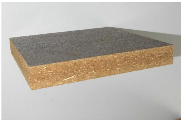
Insulation panel based on wet preserved hemp
