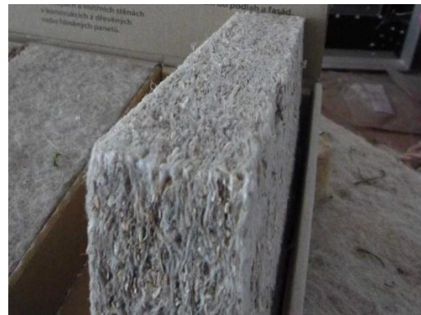
Insulation panel based on hemp fibres and shives (Canabest)
