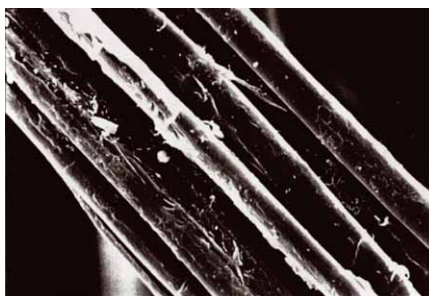
Flax fibres gained by ultrasonic treatment. Picture: ECCO
