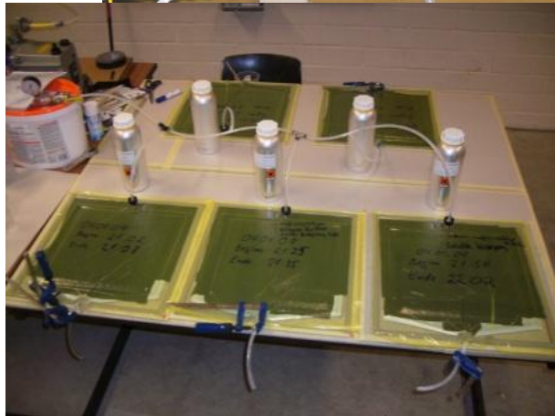
Manufacturing of test coupons
