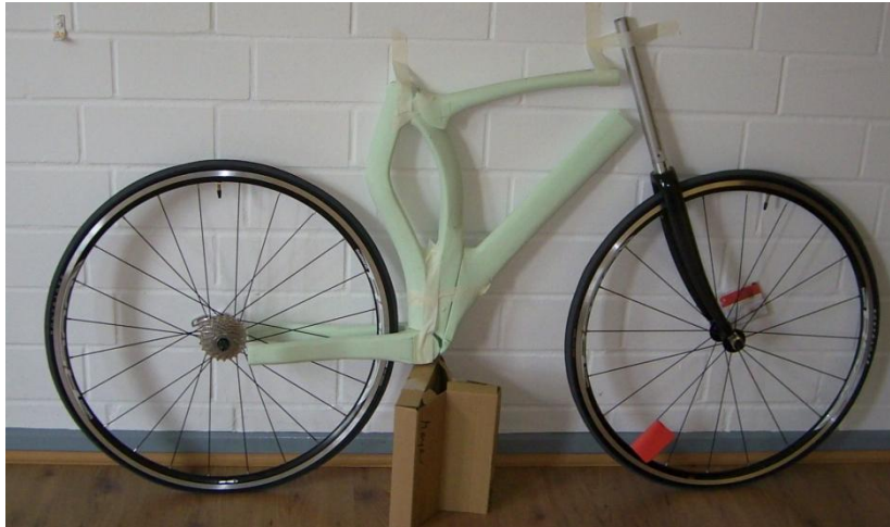
wheels an positiv mould of the frame
