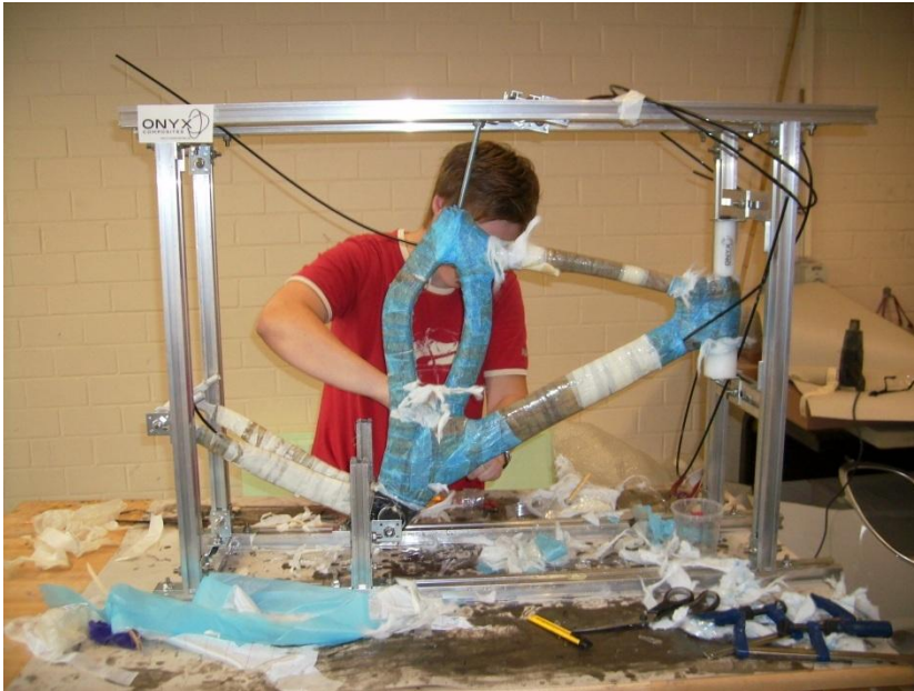
Laminating by hand with epoxiresin
