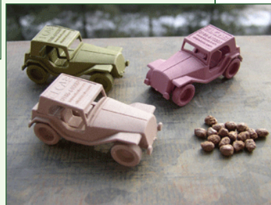
Toy Cars Made by Injection Moulding
