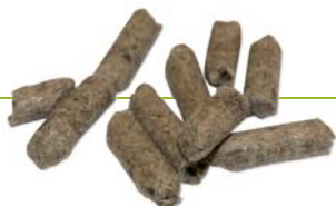
Hemp fibre pellets for granule production. Picture: nova-Institut
