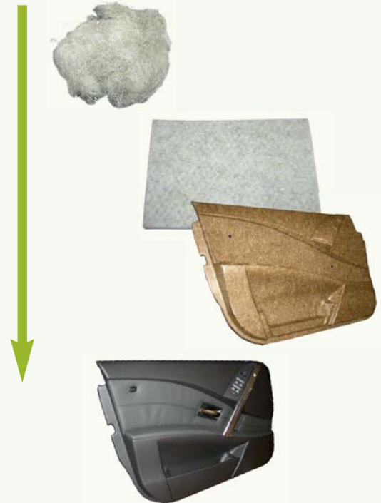
Natural fibre door panel for BMW 5 Series, compress moulding (Germany). Pictures: nova-Institut
