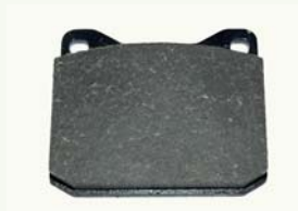
Hemp fibre brake pad for regional trains (UK). Picture: nova-Institut
