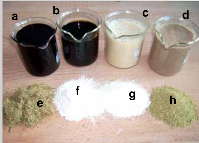
a) Phenol-Formaldehyde Resin, b) Solution of lactic acid, Glucoses, c), d) Plant rests of Glucoses production, e) Hemp fibres, f) Starch, g) Celluloses, h) canola press cake
