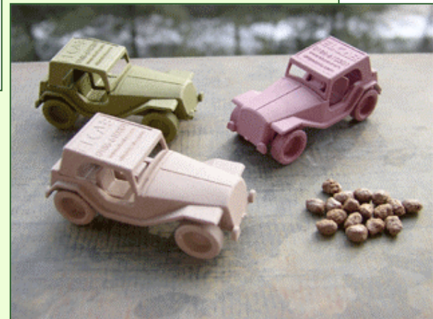
Toy Cars Made by Injection Moulding
