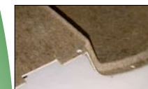
Nonwoven mat is molded into the shape of the interior trim part
