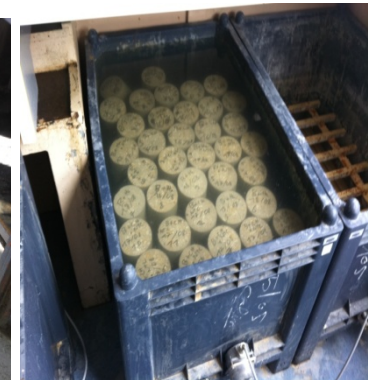
Fig Confection and conservation of samples mortar (20°C in 100% H)
