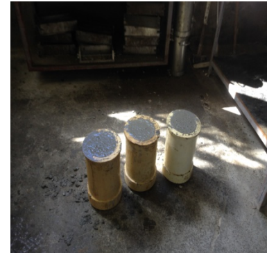
Fig Confection and conservation of samples mortar (20°C in 100% H)
