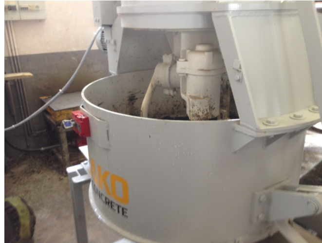
Fig Mixer of concrete
