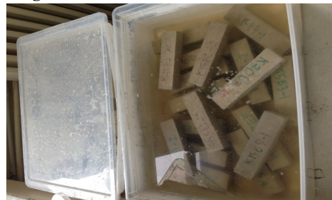
Fig Confection and conservation of samples mortar (20°C in 100% H)
