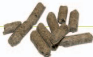
Hemp fibre pellets for granule production.
